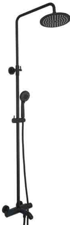
Thermostatic bar valve with 3 outlets, adjustable riser and multifunction shower handle HP 1
