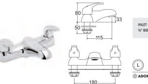
INLET CONNECTIONS: WORKING PRESSURE: 3/4" BSP 0.1 - 5.0 bar
